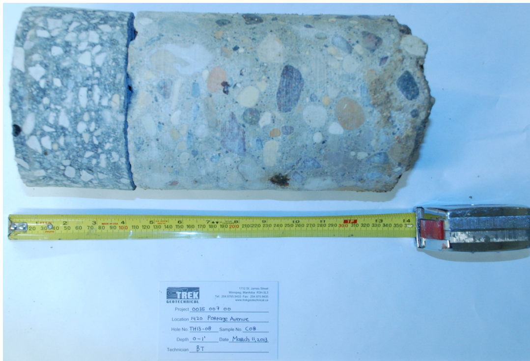
Photo 8: Asphalt and Concrete Core Sample from Test Hole TH13-08
