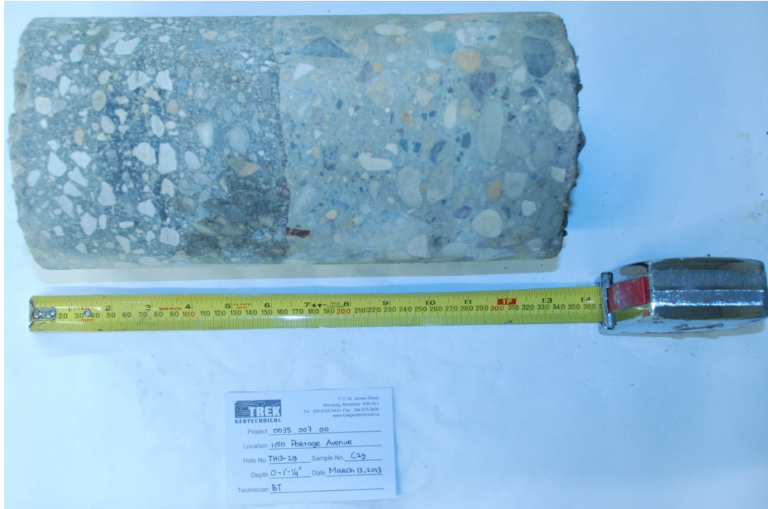
Photo 29: Asphalt and Concrete Core Sample from Test Hole TH13-29
