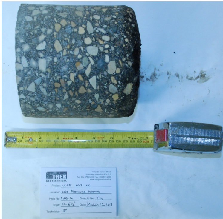
Photo 14: Asphalt Core Sample from Test Hole TH13-14
