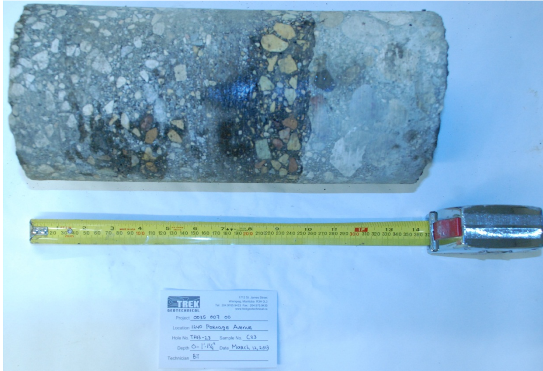
Photo 23: Asphalt and Concrete Core Sample from Test Hole TH13-23
