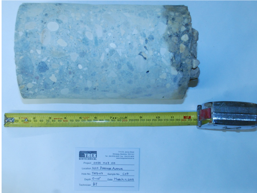
Photo 7: Concrete core sample from Test Hole TH13-07
