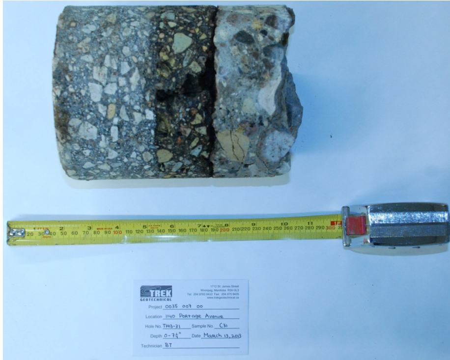
Photo 31: Asphalt and Concrete Core Sample from Test Hole TH13-31
