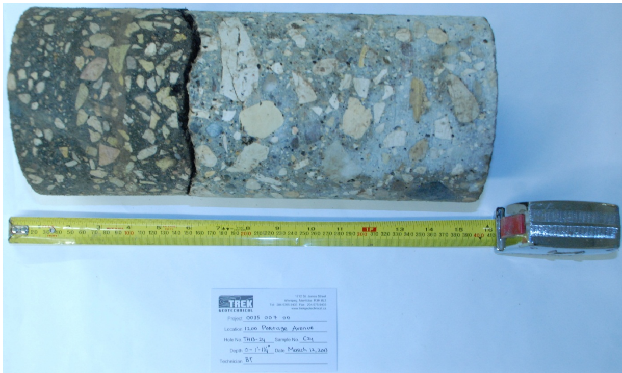
Photo 24: Asphalt and Concrete Core Sample from Test Hole TH13-24
