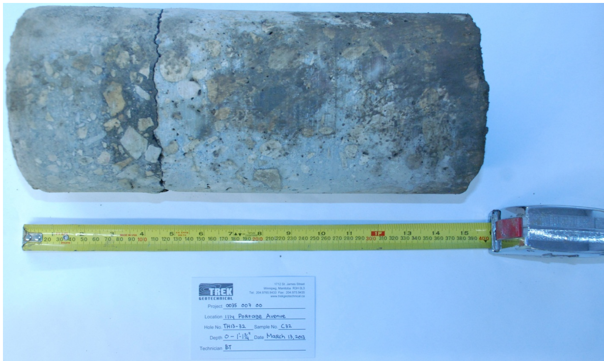
Photo 32: Asphalt and Concrete Core Sample from Test Hole TH13-32
