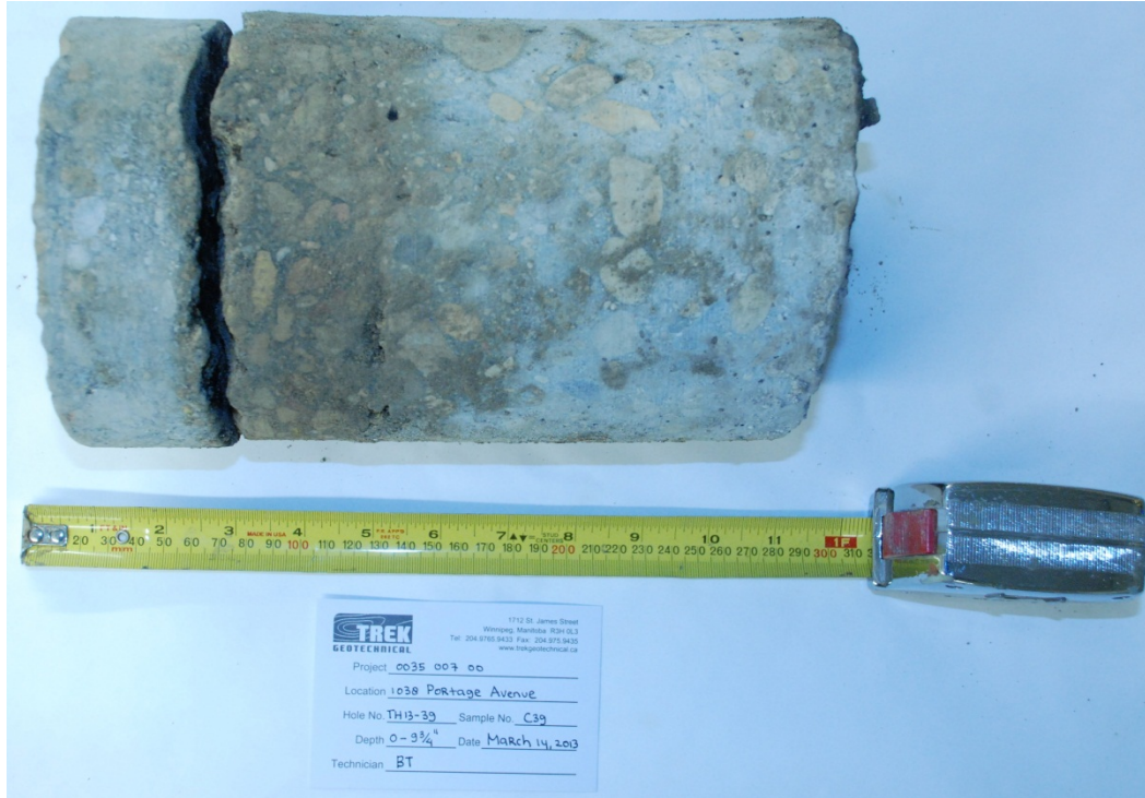
Photo 39: Asphalt and Concrete Core Sample from Test Hole TH13-39
