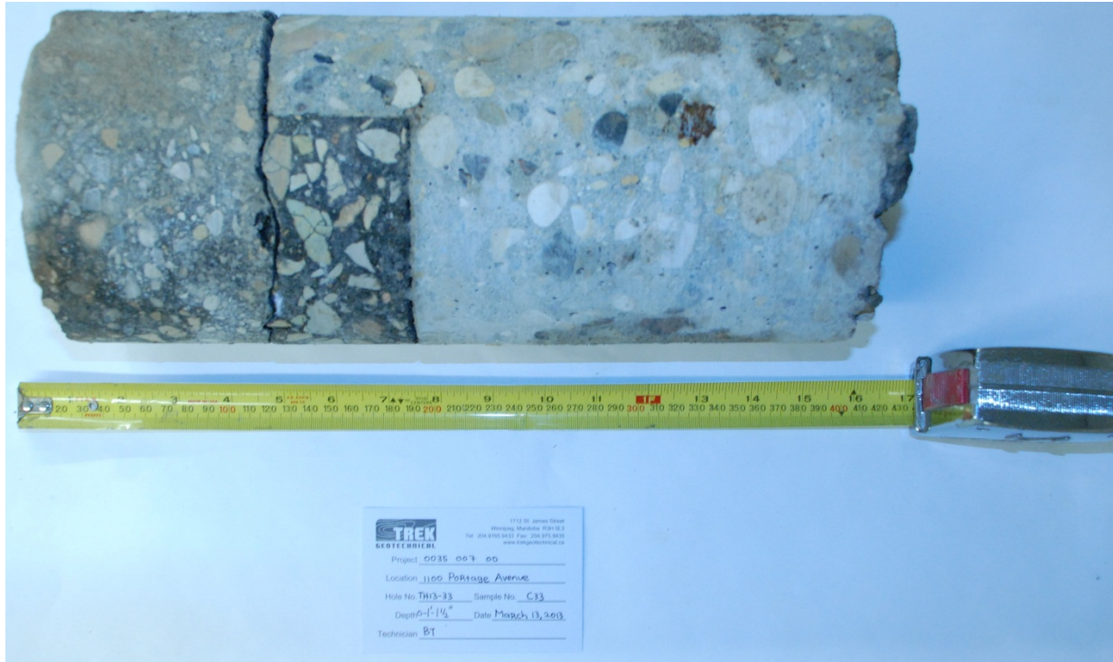
Photo 33: Asphalt and Concrete Core Sample from Test Hole TH13-33
