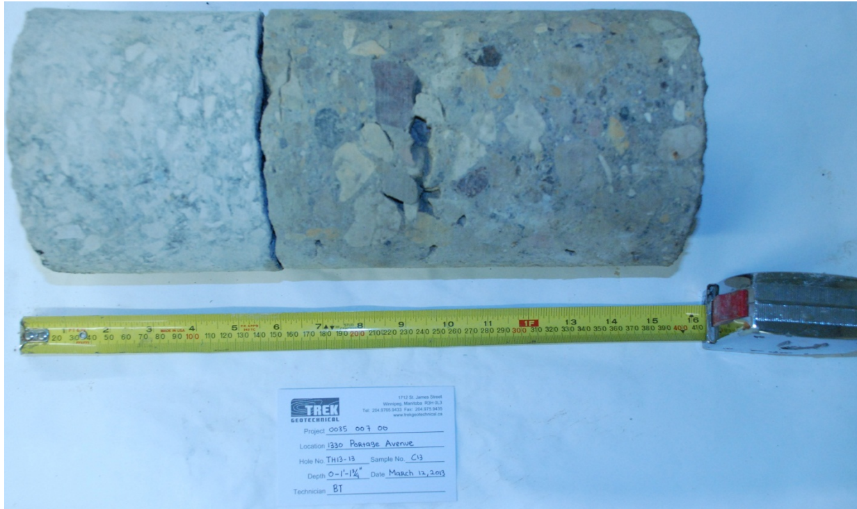
Photo 13: Asphalt and Concrete Core Sample from Test Hole TH13-13
