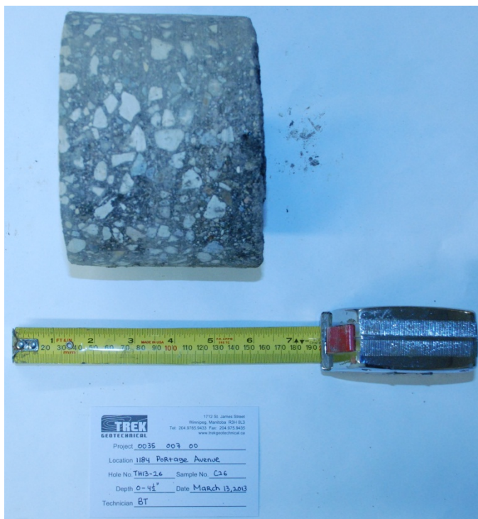
Photo 26: Asphalt Core Sample from Test Hole TH13-26
