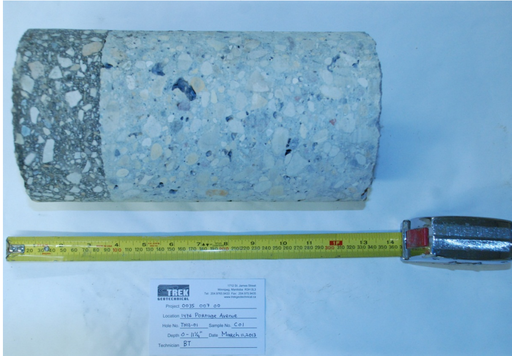
Photo 1: Asphalt and Concrete Core Sample from Test Hole TH13-01
