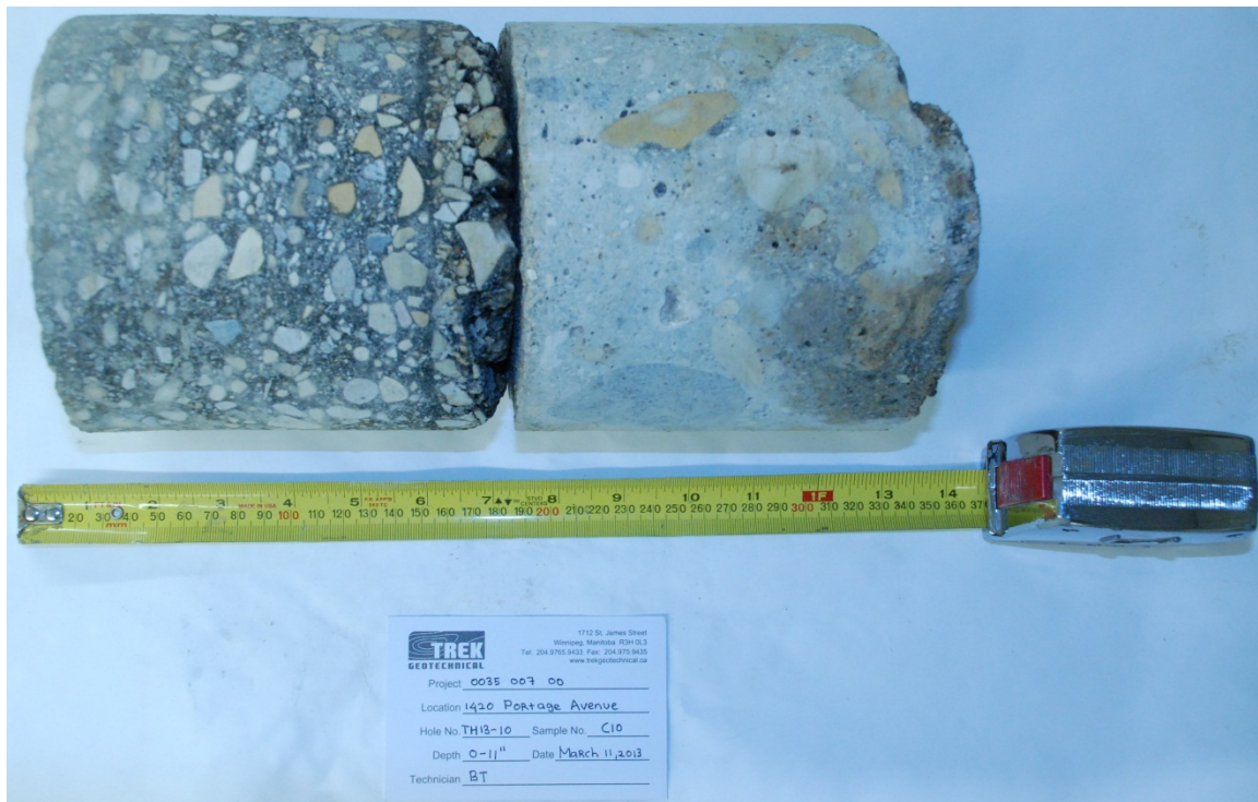
Photo 10: Asphalt and Concrete Core Sample from Test Hole TH13-10
